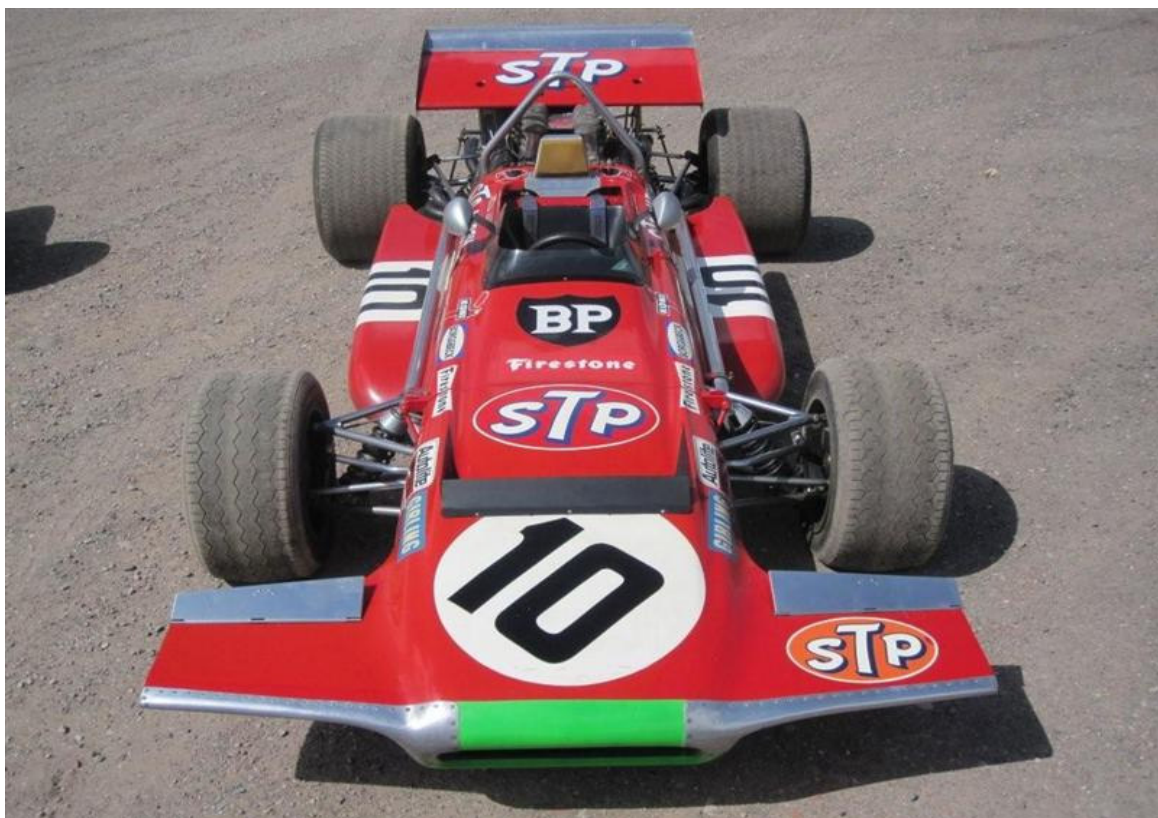
Roger Wills, UK - ex Amon 1970 March 701-1 Cosworth DFV V8 3.0 litre Formula One
